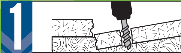
A Pattern of small holes is drilled into the sunken area.
