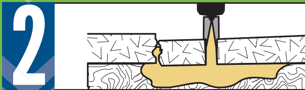
ECO-R+SE™ is pumped into the void and lifts the concrete with virtually no mess.
